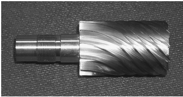
Fig. 2 Photograph of the helical swirler for the air delivery tube.
