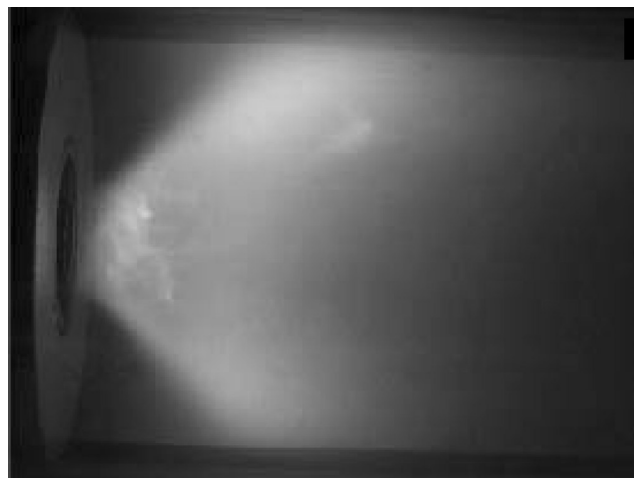
Fig. 3 Photograph of the gas-phase (methane) combustor during prototype testing (long-duration exposure). The flame is highly turbulent and lifted from the fuel delivery tube.
